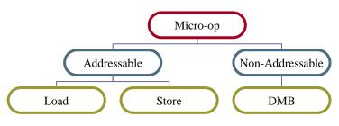
Figure 11. Typical class hierarchy of CPU instructions types
